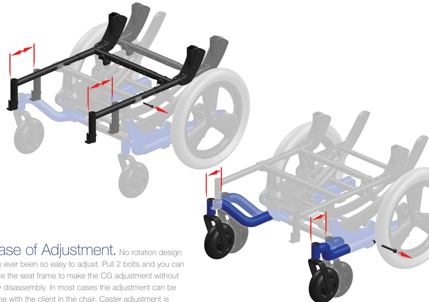
Ease of Adjustment. No rotation design has ever been so easy to adjust. Pull 2 bolts and you can slide the seat frame to make the CG adjustment without any disassembly. In most cases the adjustment can be done with the client in the chair. Caster adjustment is intuitive and again only requires you to pull 2 bolts.
